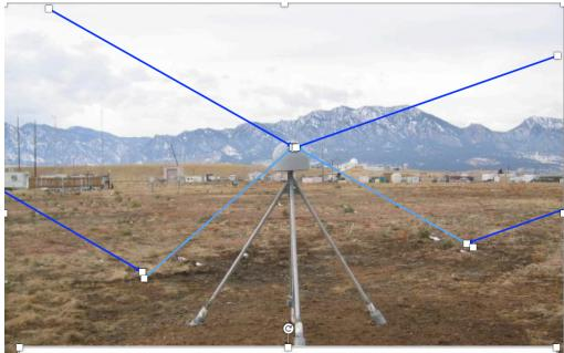
GPS Reflectometry uses the interference between direct and reflected GPS power signals to measure environmental characteristics of the reflection area, esp. the <u>height of the antenna above the reflecting surface</u>
