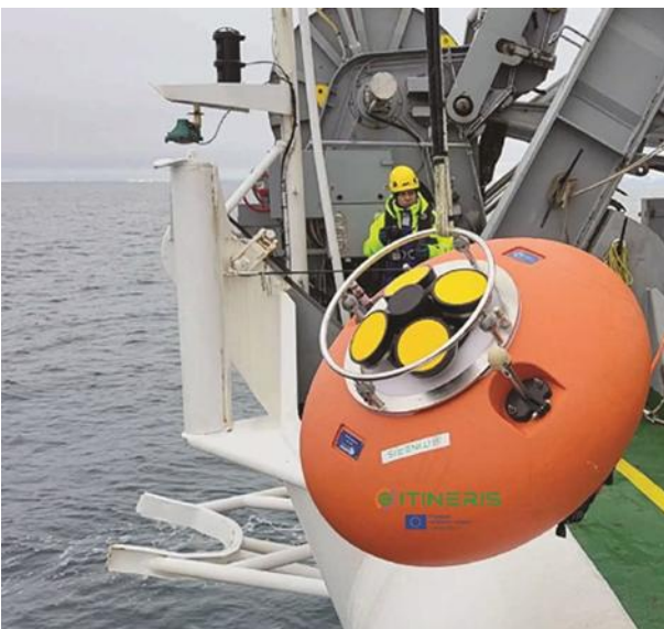
Picture 4. Deployment of an ADCP current profiler on the top-buoy of the nS1 mooring during the ACO25 oceanographic campaign. Credits: Patrizia Giordano
