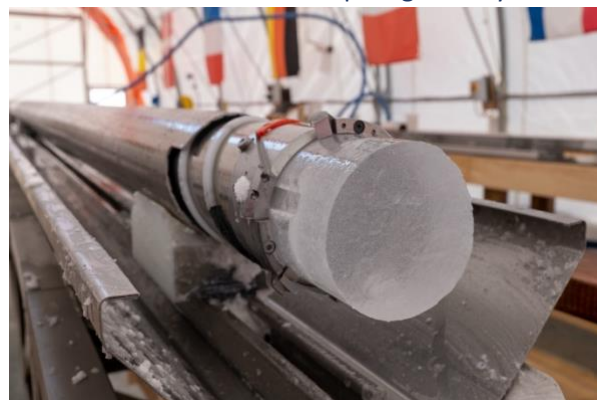
The ice core extracted from the Little Dome C site in Antarctica, visible from the head of the drill. Credits: ©PNRA/IPEV
