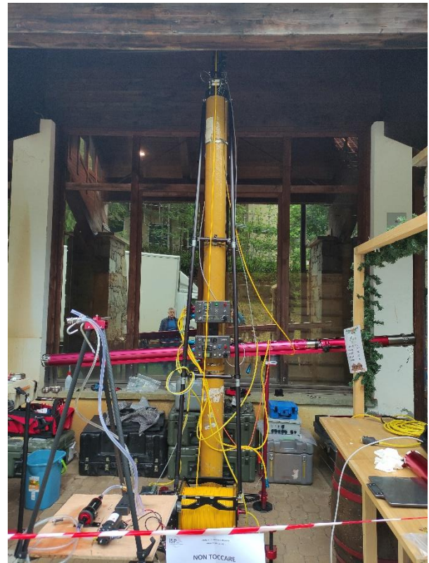
Electrothermal drill being tested in Alagna Valsesia (credits: Fabrizio De Blasi)
