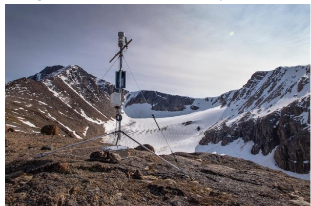
The weather station installed in late summer 2023 in the Aqqutikitsoq mountains at 840 m altitude as part of the LOGS project
