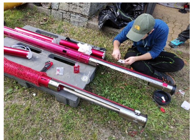
Electrothermal drill assembly (credits: Fabrizio De Blasi)
