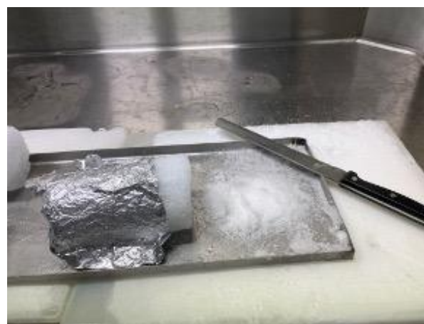
Cut and processing of the ice core. Credits: Giulia Genuzio
