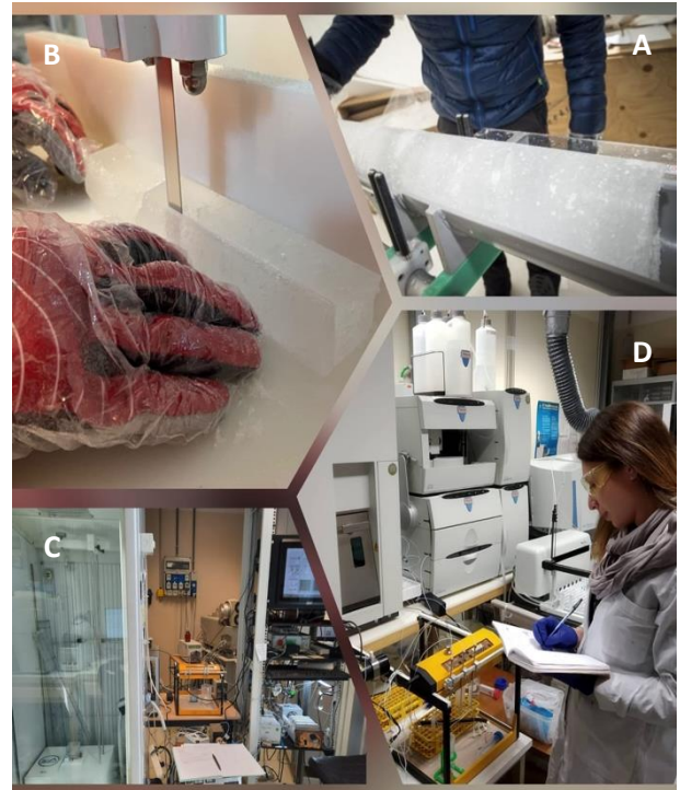
A) longitudinal view of an alpine ice core (Ph. Riccardo Selvatico); B) ice sticks (bags) cutting for CFA; C) general view of the melting system (CFA); D) coupling test phases
