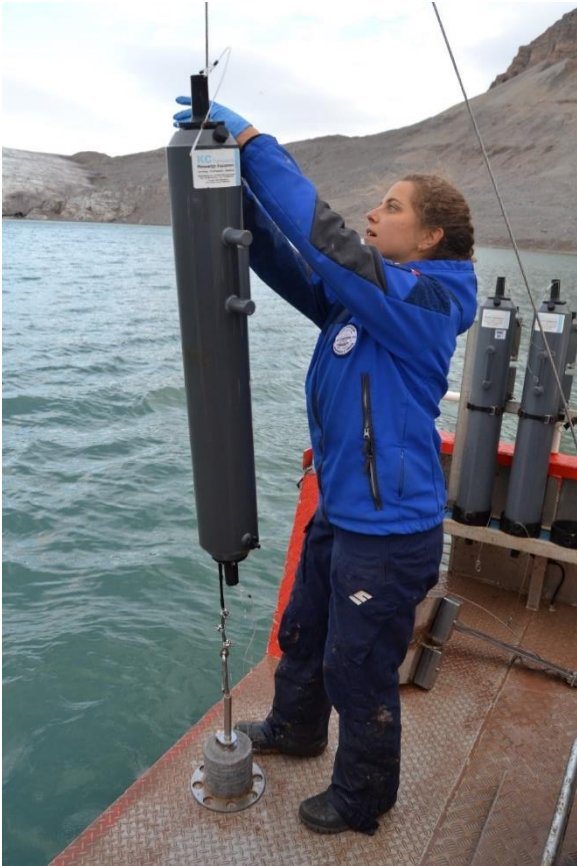
Sampling of superficial seawater with the Niskin bottle in Kongsfjorden (Svalbard Archipelago). Credits: Sara Giansiracusa
