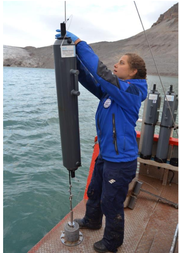
Surface water sampling by Niskin bottles on board the MS-Teisten. Credit: M. Sabino - ISP
