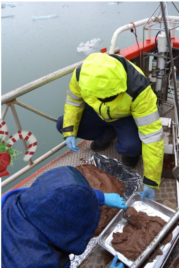
Marine sediment sampling by bucket aboard KingsBay's MS Teisten. Credit: S. Giansiracusa - ISP
