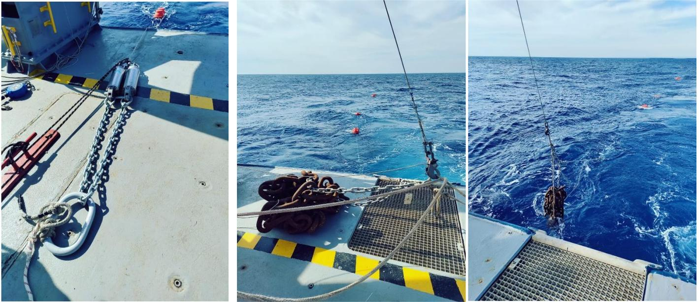
**Figure 10.-** Mooring ballast and release system before final launch
