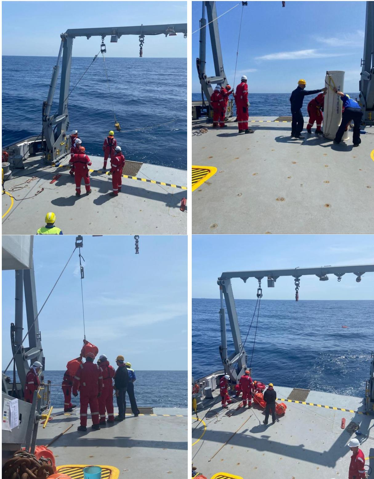
**Figure 8.-** Phases of mooring FF recovery
